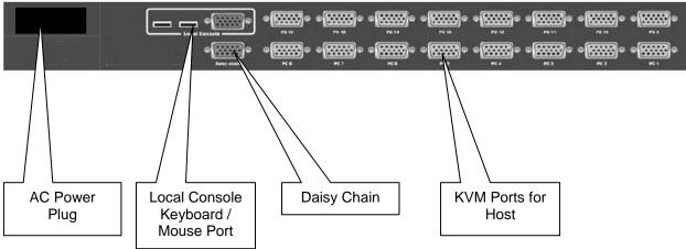
3.2 Connecting KVM Ports for Host using PS/2 connection. Connect single ended D-Sub end to KVM port and other end composing of VGA D-Sub, PS/2 Keyboard (Green) and PS/2 Mouse (Purple) to corresponding ports on the system.
