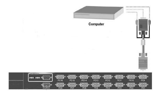
3.3 Connecting KVM Ports for Host using USB connection. Connect single ended D-Sub end to KVM port and other end composing of VGA D-Sub and USB to corresponding ports on the system.
