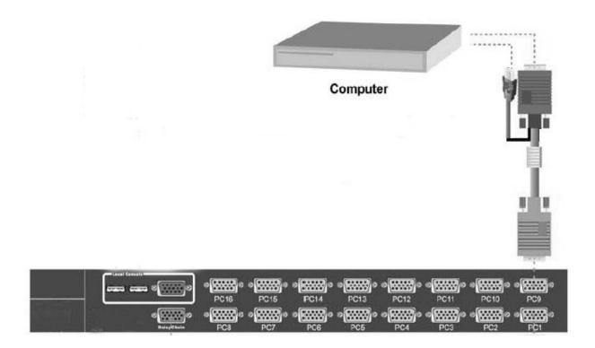
3.4 You can connect a local console port to operate the KVM bypassing the built-in LCD and keyboard/touchpad through the rear local console port. Connect the VGA D-Sub connector and USB keyboard and USB mouse to the port marked. \*\*On 980P/990P, USB is replaced with PS/2 connectors.
