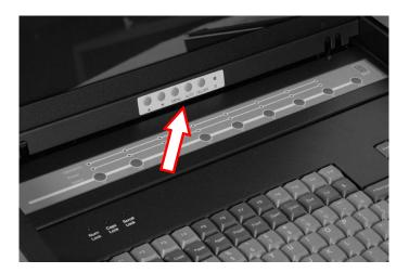
6.2 Adjust LCD OSD to match the display to your video board via the OSD button located on right side of the LCD panel. Press the MENU button to bring the on screen menu out and then follow instructions. Press the UP/DOWN button to scroll through the menu and press the SELECT button to enter the selected item. And UP/DOWN button to adjust value as necessary.
