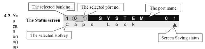
the KVM OSD by pressing the **Cap Lock** key <u>twice</u> and then **Space Bar**. \*For 980P/990P, the sequence will be **Scroll Lock** key **twice** and the **Space Bar**.
