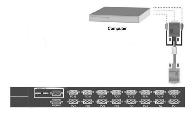
3.3 Connecting KVM Ports for Host using USB connection. Connect single ended D-Sub end to KVM port and other end composing of VGA D-Sub and USB to corresponding ports on the system.
