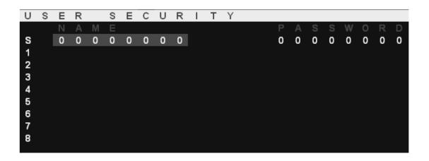
Press the **Enter** key or left button of mouse for editing. The left-top "S" means SUPERVISOR, and "1", "2", "3",..., "8" mean USERs. The maximum length of NAME and PASSWORD is eight characters (A~Z and 0~9).
