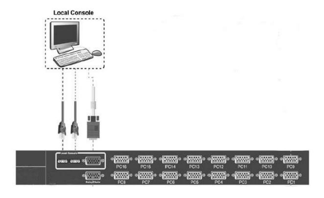
3.5 You can connect additional KVM port by adding additional KVM switches and connecting between them a daisy chain cable. The control will be from the primary KVM by changing banks selection.
