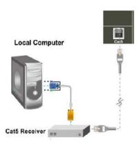
3.7 Optional IP Remote Console Module Available for allow redirect of keyboard, mouse and mouse data to a remote administration console. It allows you to control one or many computer locally at the server site or remotely via the Internet using standard browser.
