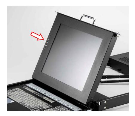
2.10 To return the drawer back to the unit, fold screen down and push in the 2 tap located on each side of the rail then push the drawer back in.
