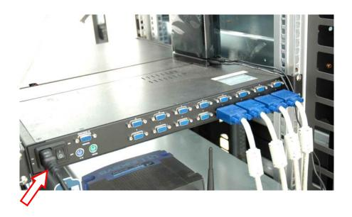
2.5 Connect the host cable to the rear of the drawer. For the 920U, USB type can be connected to its single port. For 980D/990D both PS/2 and USB type can be use with the KVM, just choose the desire type to match with your system, the KVM accepts both. Refer to **Section 3** for further detail. (\*980 Shown)
