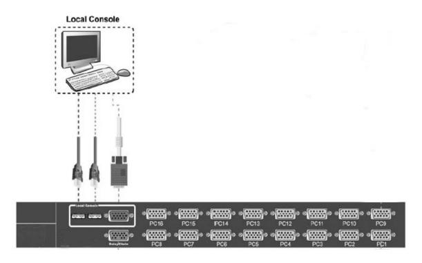
3.5 You can connect additional KVM port by adding additional KVM switches and connecting between them a daisy chain cable. The control will be from the primary KVM by changing banks selection.
