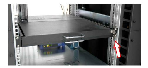
2.8 Once the drawer is fully extended, lift up the LCD panel and tilt back, this will allow you to view the LCD and access the keyboard/touchpad.
