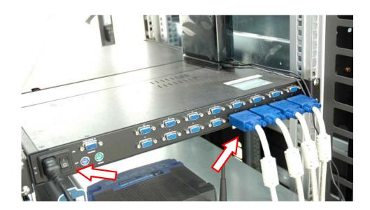
2.6 You can turn on the drawer unit main power on the back of the chassis.
