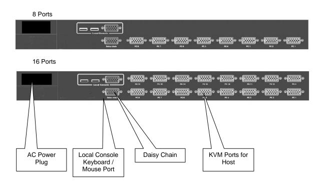
3.2 Connecting KVM Ports for Host using PS/2 connection. Connect single ended D-Sub end to KVM port and other end composing of VGA D-Sub, PS/2 Keyboard (Green) and PS/2 Mouse (Purple) to corresponding ports on the system.
