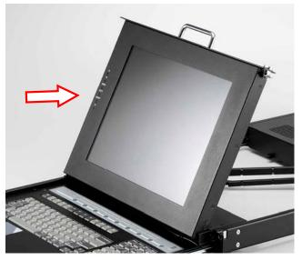
6.2 Adjust LCD OSD to match the display to your video board via the OSD button located on right side of the LCD panel. Press the MENU button to bring the on screen menu out and then follow instructions. Press the UP/DOWN button to scroll through the menu and press the SELECT button to enter the selected item. And UP/DOWN button to adjust value as necessary.
