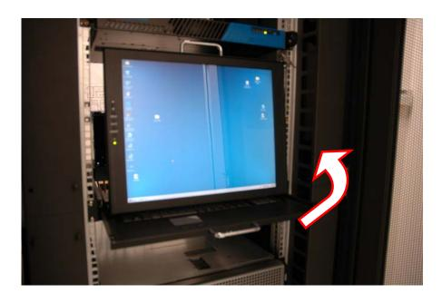
2.9 To turn on the power for the LCD panel, the power button located beneath the LCD can be use to independently turn on/off. LCD screen adjustment button is also located here.
